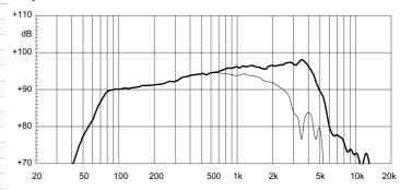
FREQUENCY RESPONSE CURVE OF 8NMB420 MADE ON 25LIT. ENCLOSURE TUNED 65HZ IN FREE FIELD (4PI) ENVIRONMENT. ENCLOSURE CLOSES THE REAR OF THE DRIVER. THE THIN LINE REPRESENTS 45 DEG. OFF AXIS FREQUENCY RESPONSE FREE AIR IMPEDANCE MAGNITUDE CURVE
