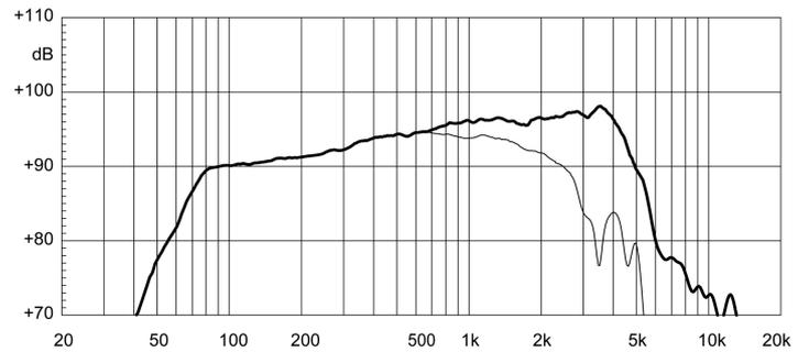
**FREQUENCY RESPONSE CURVE OF 8NMB420 MADE ON 25LIT. ENCLOSURE TUNED 65HZ IN FREE FIELD (4PI) ENVIRONMENT. ENCLOSURE CLOSES THE REAR OF THE DRIVER. THE THIN LINE REPRESENTS 45 DEG. OFF AXIS FREQUENCY RESPONSE FREE AIR IMPEDANCE MAGNITUDE CURVE**
